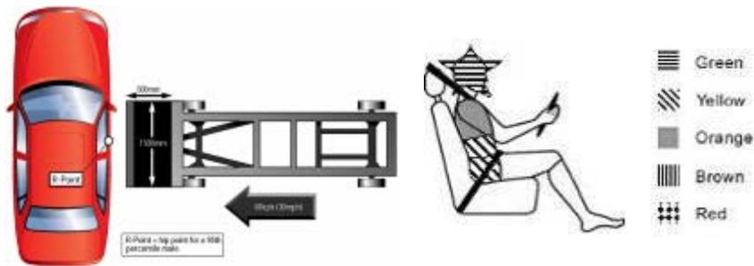
Figure 2- Side crash test procedure and color scale for the driver.
